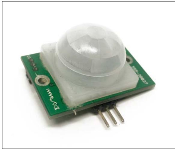
Here, I used a very simple PIR motion detector. This sensor will measure the infrared (IR) light that is emitted by moving objects in its field of view, for example, people moving around. It is really easy and quite cheap to interface with Arduino. You can use any brand that you want for this sensor; it just needs a voltage level of 5V in order to be compatible with the Arduino Uno board.
