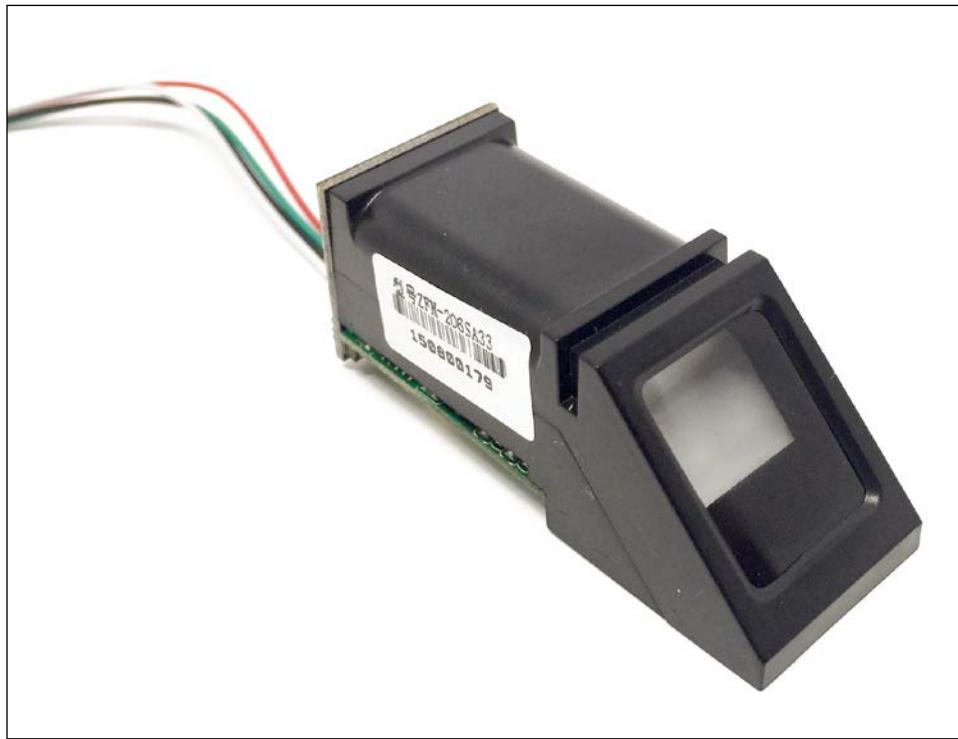
You will need a fingerprint sensor: software requisites "need to get with fingerprint sensor: hardware requisites" the exact same model (from Adafruit). Otherwise, the code for this project won't work.
