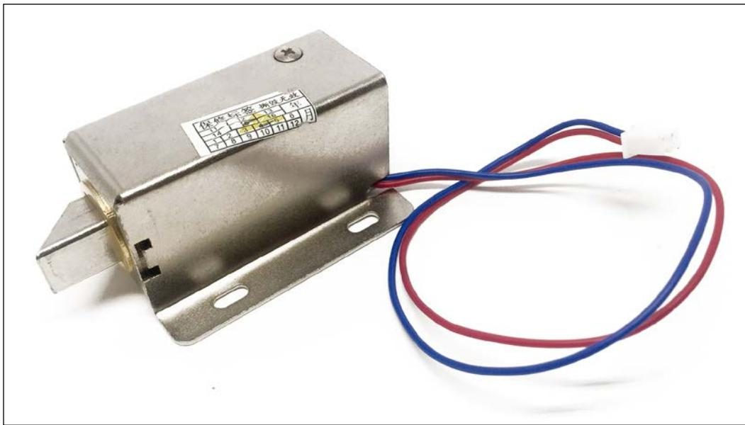
First, you'll need to cut the JST connector from the electronic lock in order to be able to connect it to the breadboard. I soldered some 2-pin header at the end of the electronic lock to make it compatible with my breadboard.
